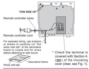
\* If the Y-shaped terminal is not covered, the exposed section may come into contact with the mounting bracket resulting in improper operation or failure.
